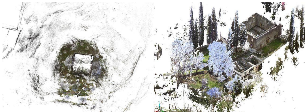
Figure 3: Laser scanning survey. Point clouds of the hammam and the part of the complex
