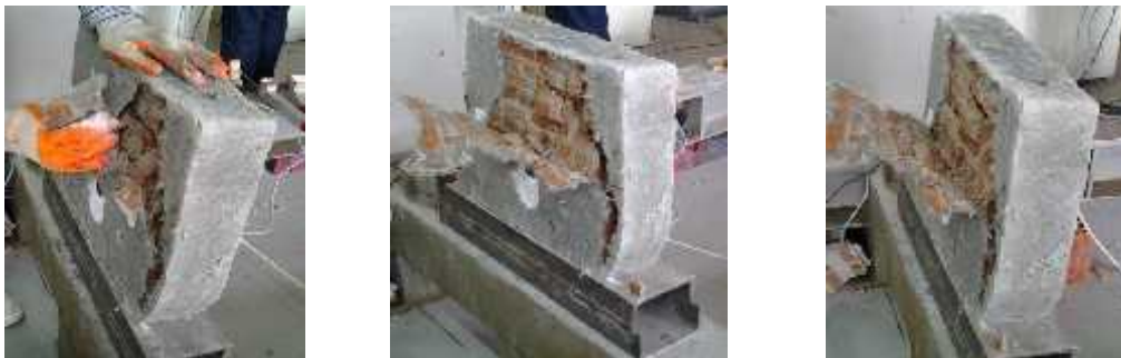
Figure 5 The polypropylene fiber plaster sample failure
