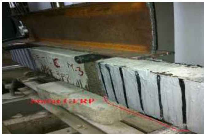
Fig.5.6 Cracks in Set C/beam 3
