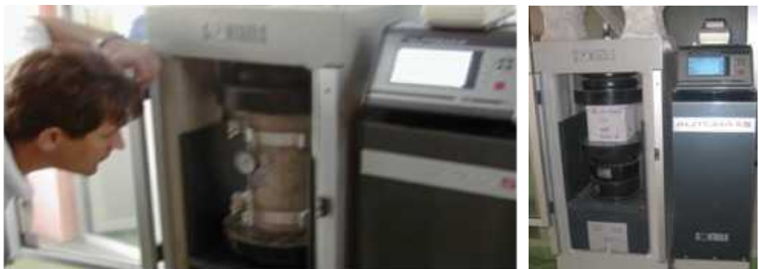
Fig.2. Testing of modulus of elasticity
