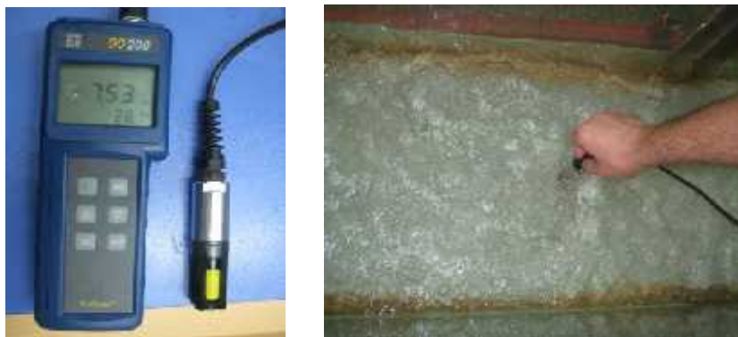
Fig. 4. A photograph of DO200 oxygen meter and dissolved oxygen measurement.
