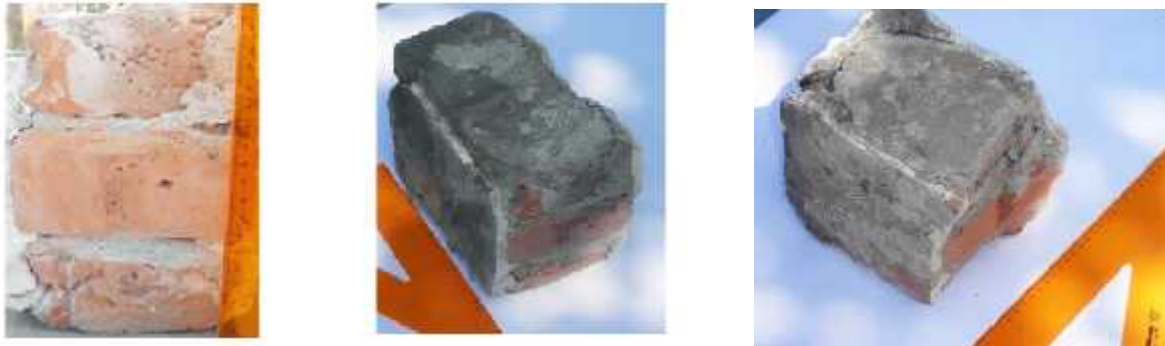
Figure 4 Masonry wall specimens
