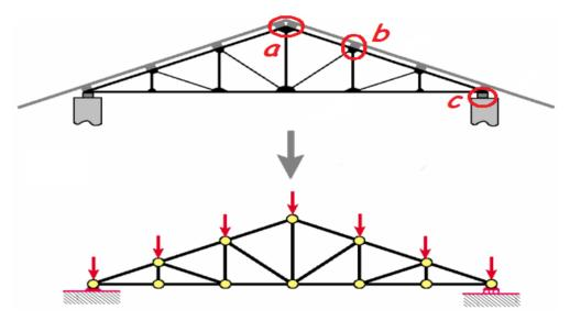
Figure 2 Roof structure and its idealization model
