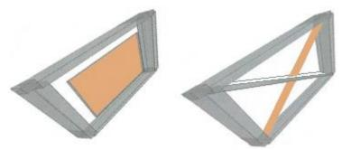
Figure 5 Timbers to braced frame
