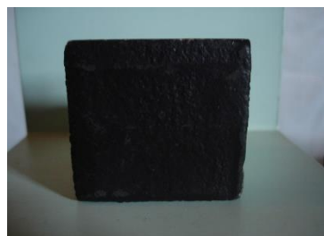
Figure 5 Ceracoat, a barrier sheath
