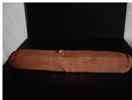
Figure 7 Water repellent adobe
