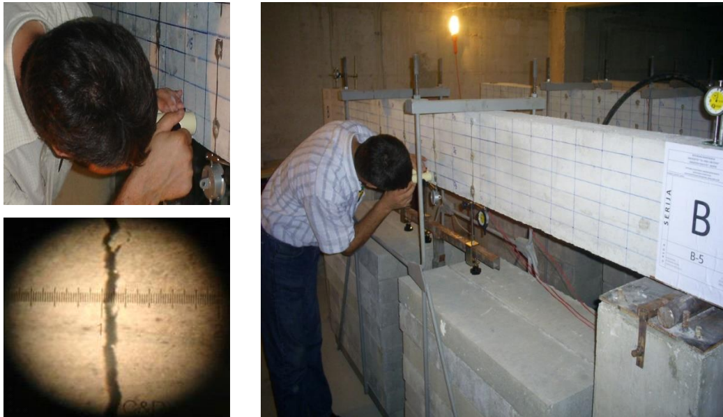
Fig. 2. Measurement process of the crack with on the beams [1].
