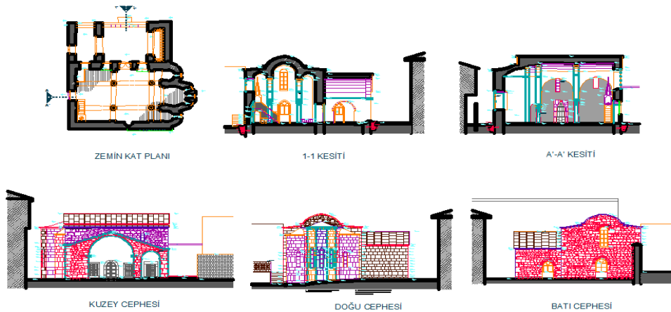
Fig. 4. Layout, inside and outside of the restoration project of Molla Siyah Mosque [20]
