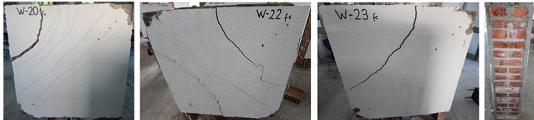
Figure 32. Failure mode of Ferrocement jacketing strengthened wall panels of Series2.
