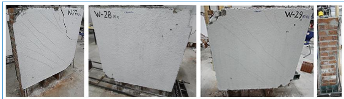
Figure 38. Failure mode of ferrocement jacketing repaired wall panels of Series 2.
