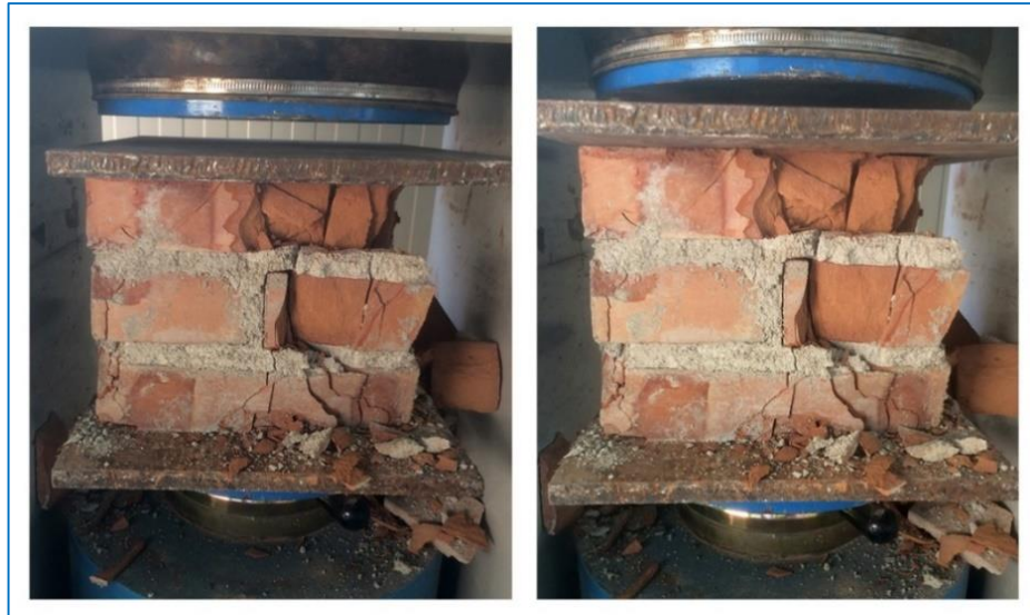
Figure 28. Determination of masonry assemblage compressive strength.
