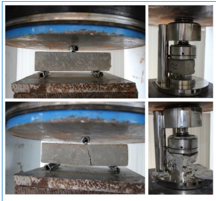
Figure 27. Determination of mortar's flexural and compressive strength.
