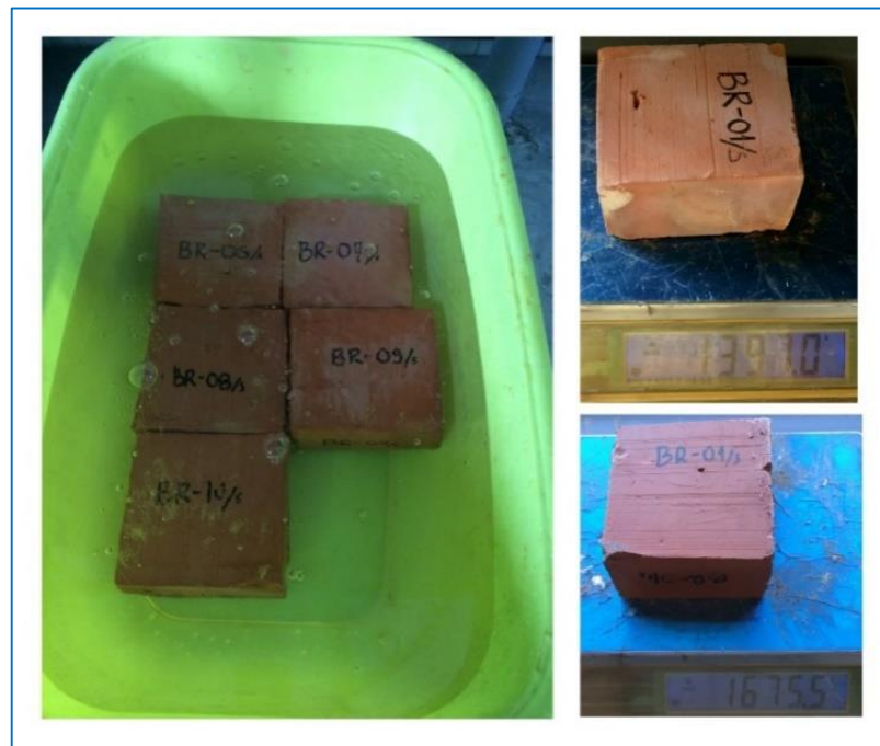
Figure 26. Determination of brick water absorption.
