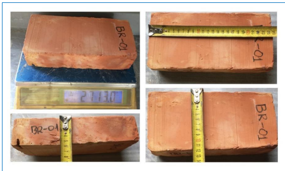
Figure 25. Determining brick dimensions.
