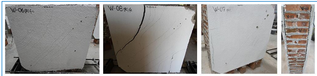
Figure 37. Failure mode of ferrocement jacketing repaired wall panels of Series 1.
