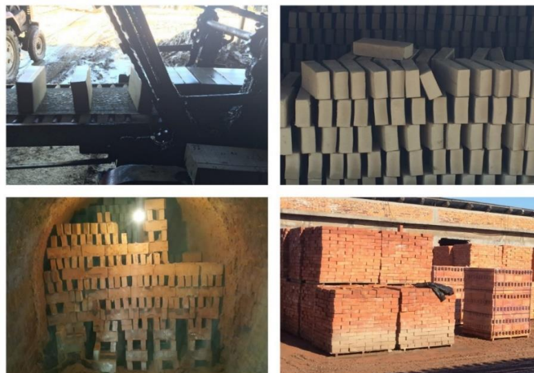
Figure 2. Air-drying, firing of bricks and the finished product ready for transport (Location: Fier, Albania).
