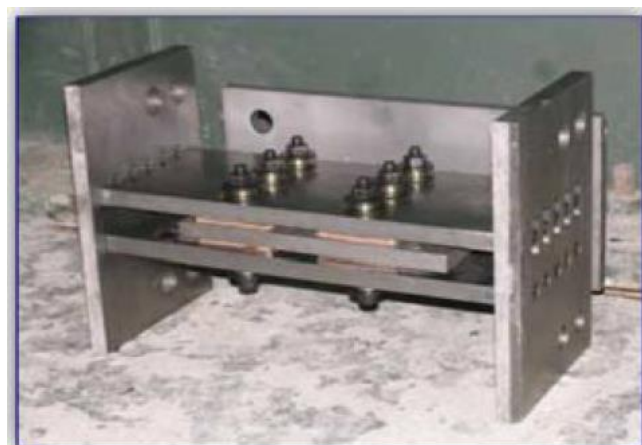
Figure 4 Slotted Bolted Connection (SBC)
