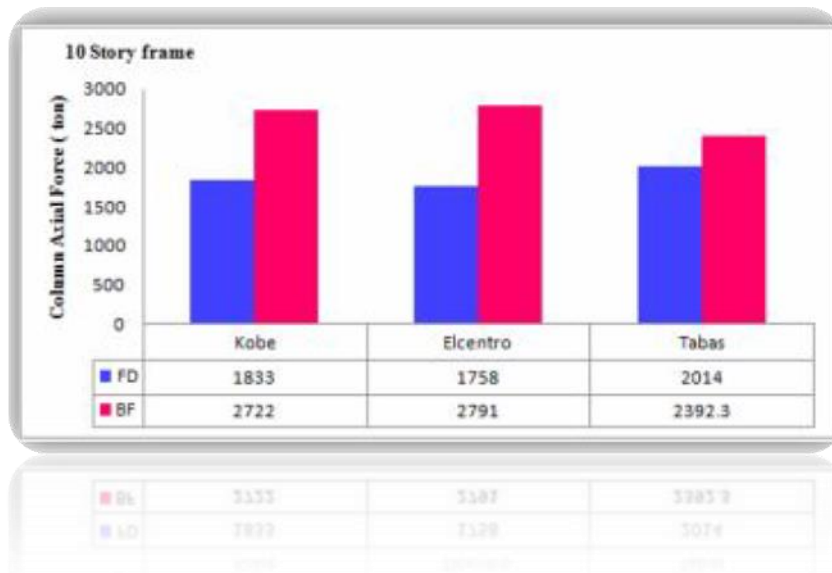
Figure 7 Envelope of Column axial force, (Vaseghi, J. et al. 2009)
