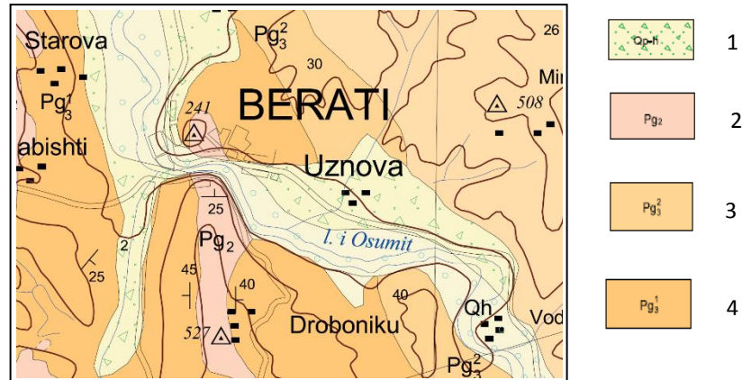
Figure 20. Quaternary deposits, alluvial and diluvium soils, 2. Eocene deposits-limestone, 3 and 4. Lower-Medium Oligocene deposits-Flysch rocks, [24]
