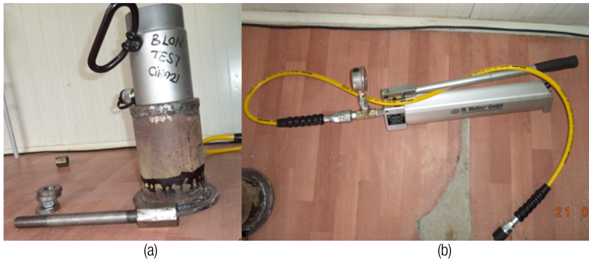
Figure 5. Rock bolt pulls out test apparatus.
