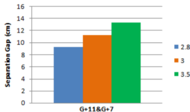
Figure 4. Variation of Separation Gap with Story Height
