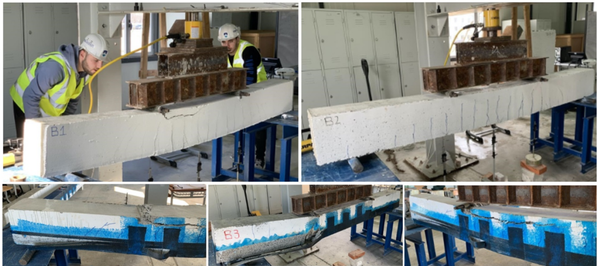
Figure 9. All the beams after failure.
