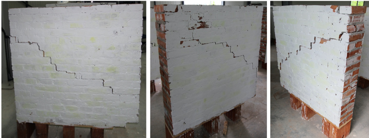
Figure 4. Failure mode of the unreinforced panels.
