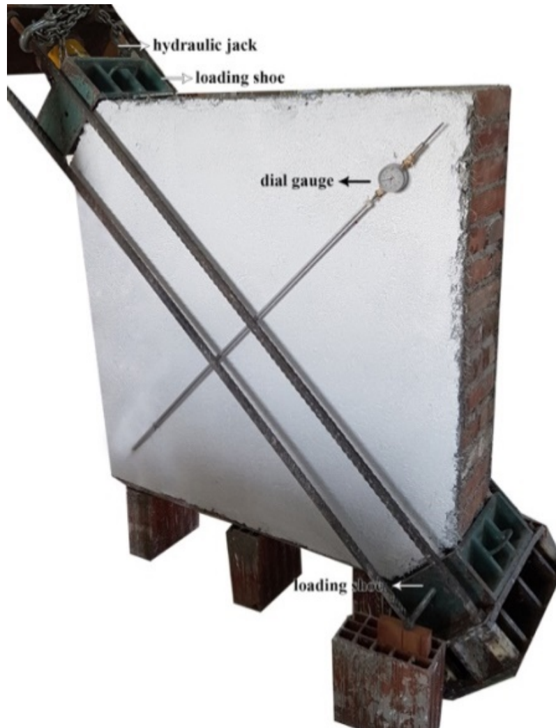
Figure 2. Diagonal compression test set-up.
