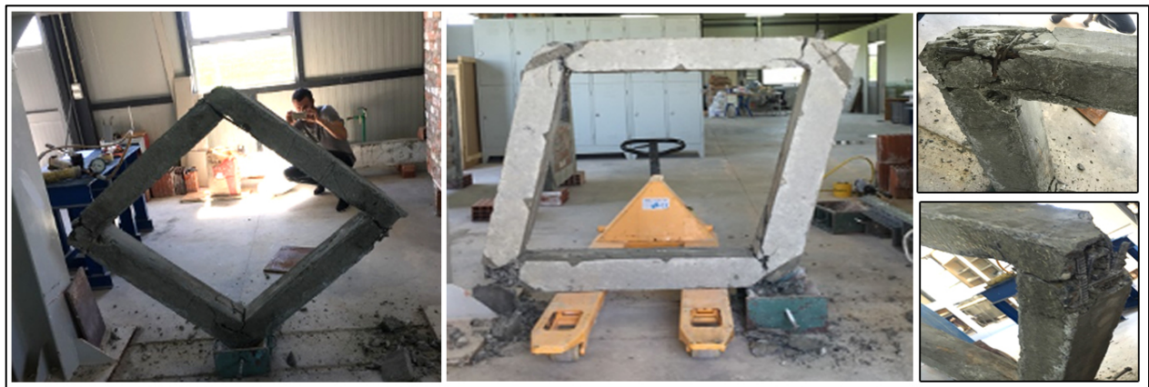
Figure 4. Deformed RC frame after the test and details of cracked joints.
