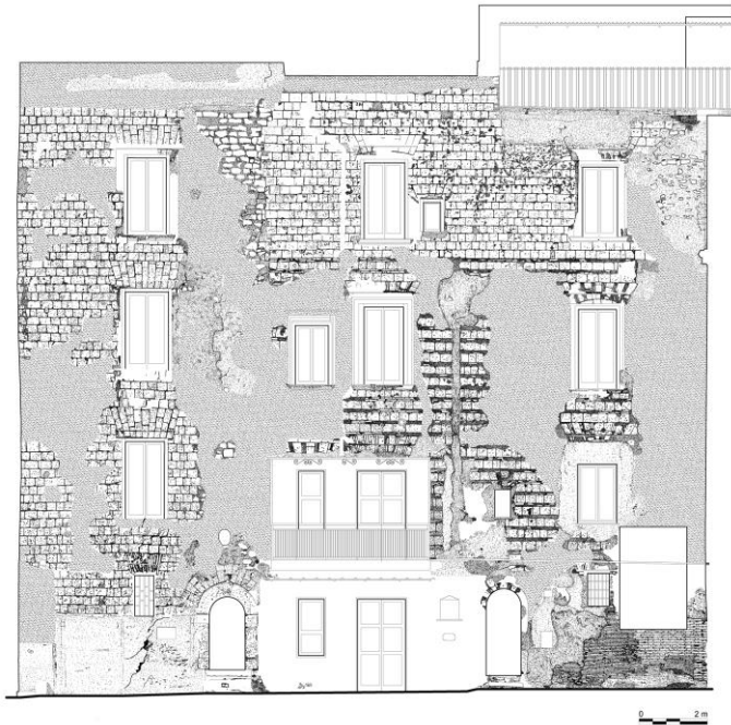
Figure 4: Napoli, building in Vico Lungo Tre Regine, material survey of a stratified façade with masonries of various construction techniques.
