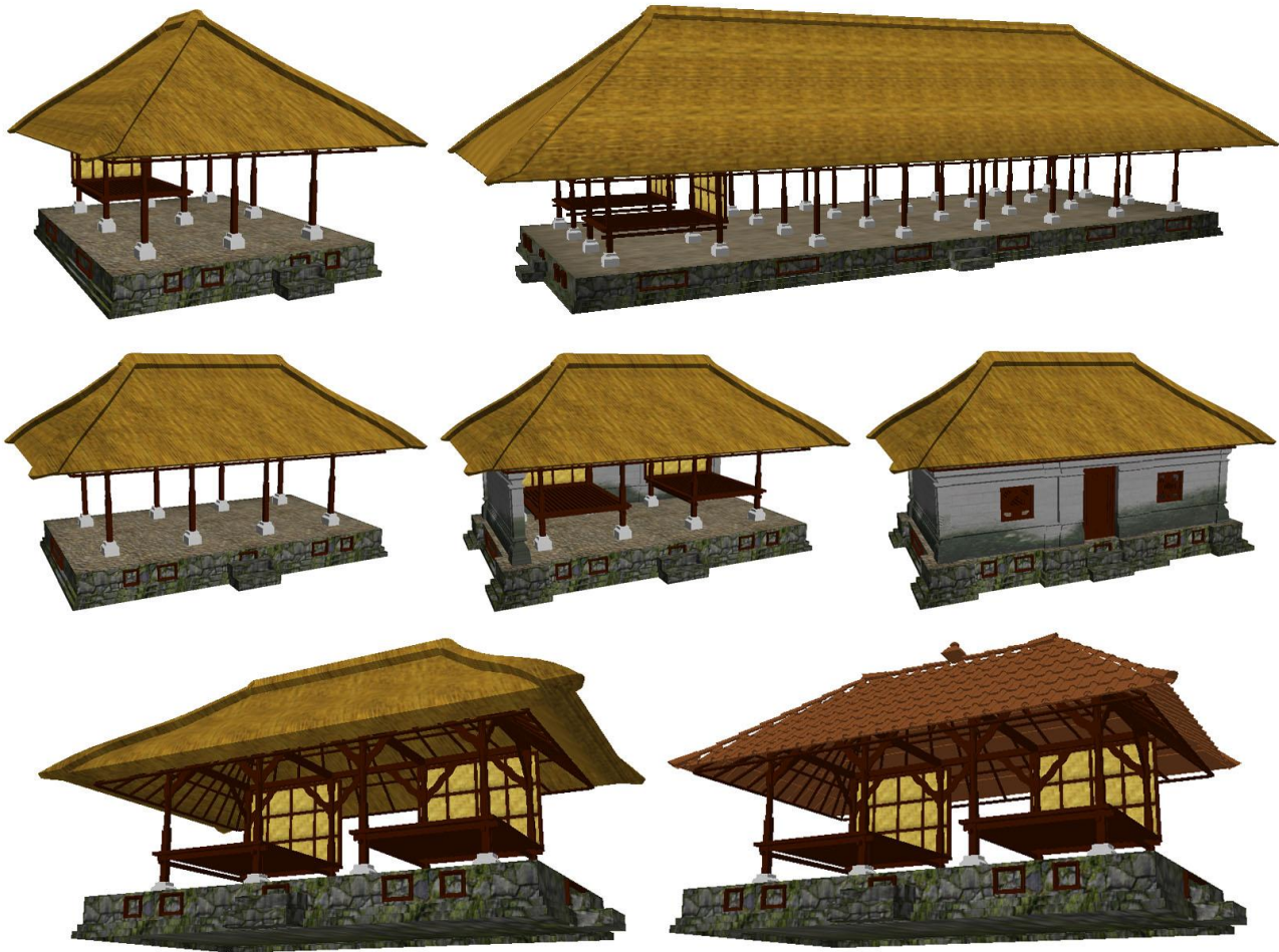
Fig. 9: (top row): Automatic placement of columns according to basement size and type of pavilion (middle row): Variants of pavilions (open, half open or closed) (bottom row): Variation of roof construction (natural grass and brick tiles)
