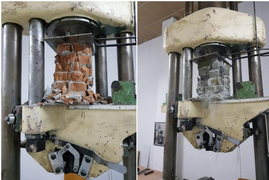
Figure 51: Masonry prism failure
