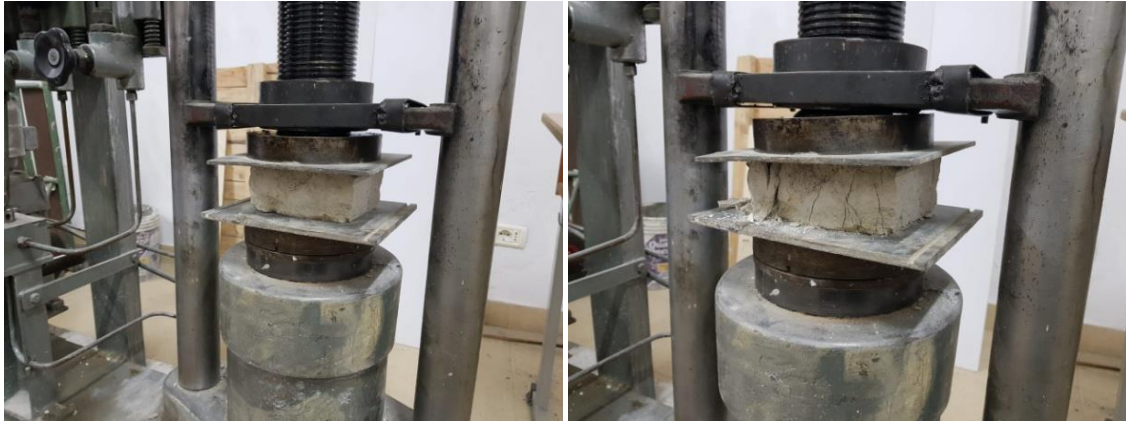
Figure 47: Brick compression test
