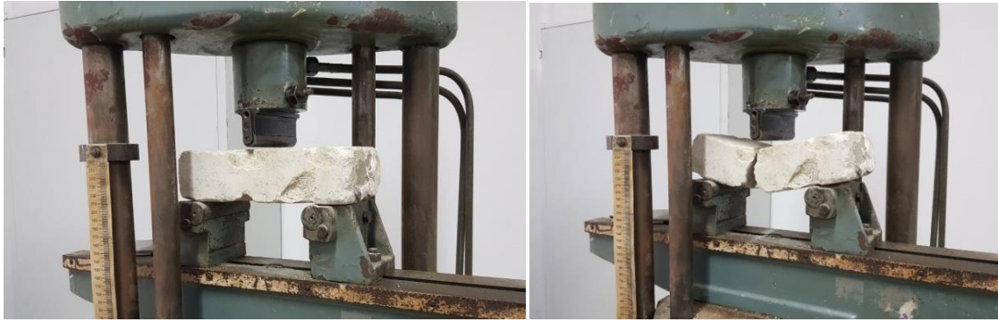
Figure 48: Tensile flexural tests and failure mechanism of solid clay bricks
