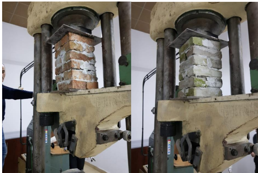
Figure 50: Specimens of prism clay masonry (left), silicate masonry (right)
