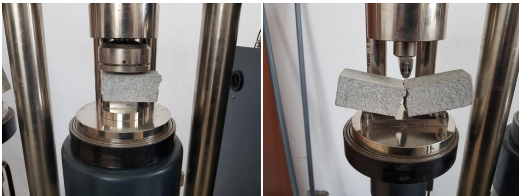
Figure 49: Compressive (left) and flexural (right) strength tests of mortar samples
