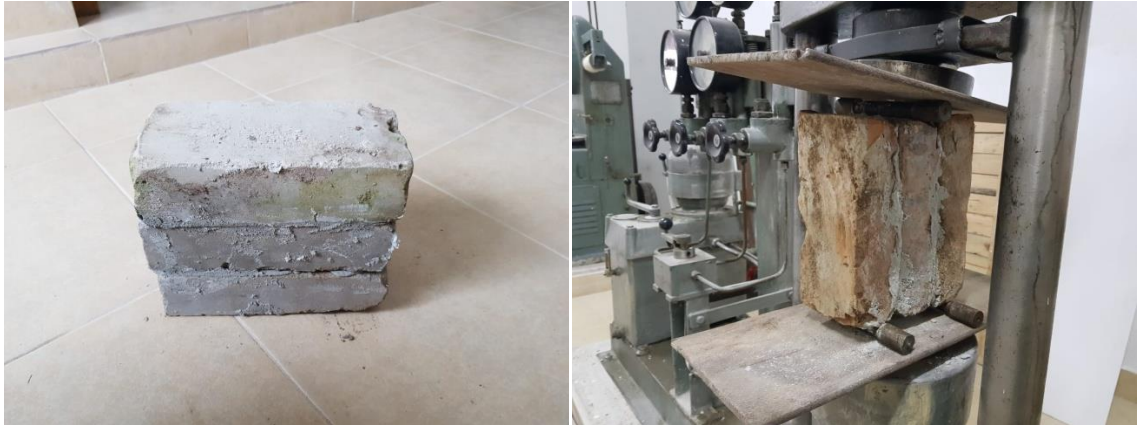
Figure 52: Masonry triplet specimen and test procedure
