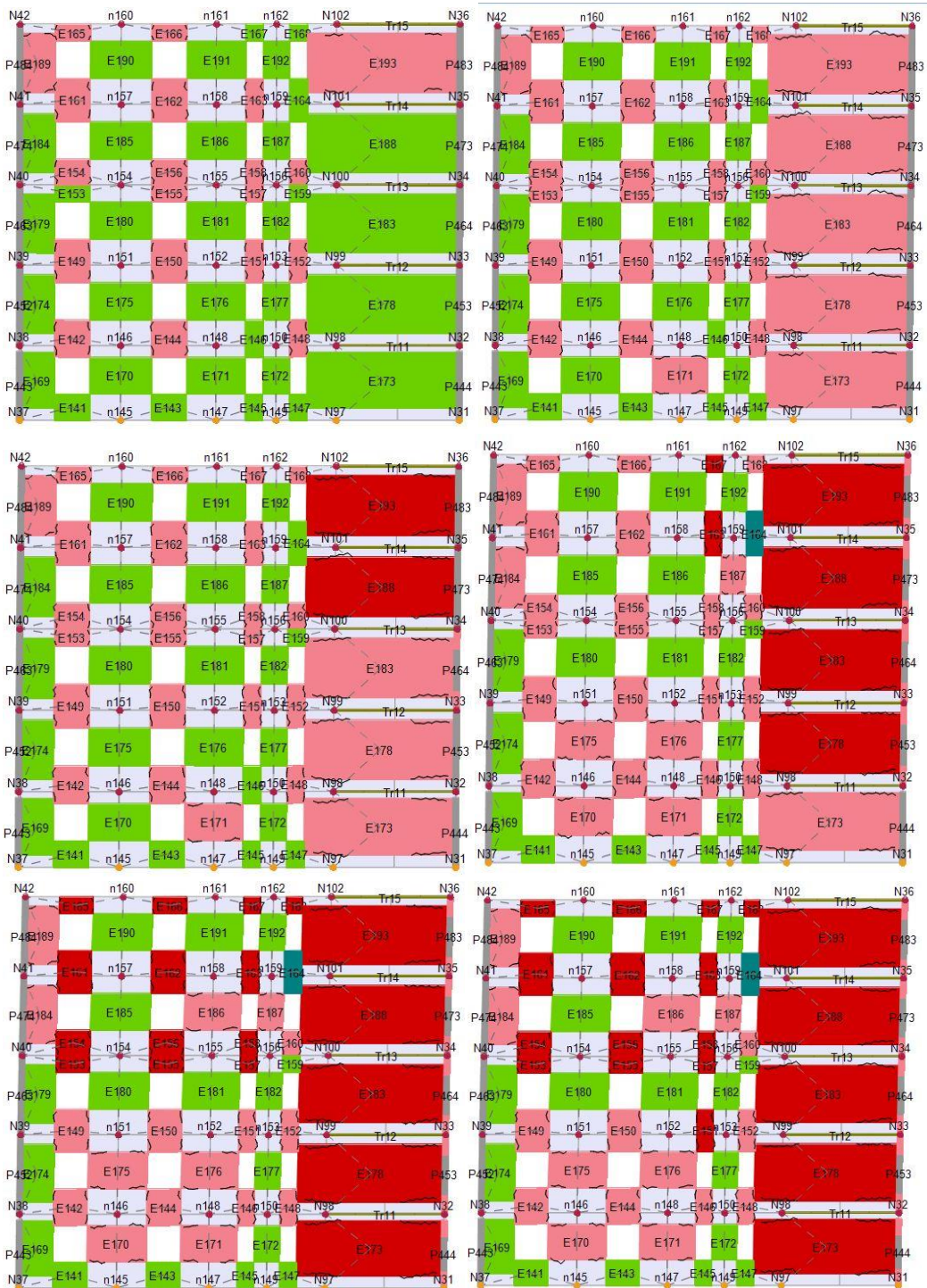
Figure 186: Perimeter wall failure mechanism C1A clay building step by step
