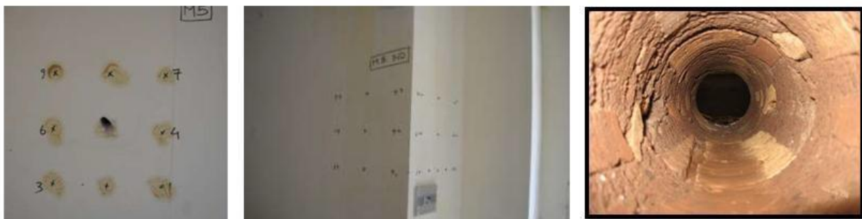
Figure 4: NDPT at Palazzo Camponeschi carried in Direct mode (left) and indirect angled mode (middle).
