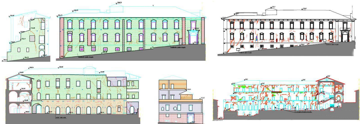
Figure 5: Different masonry types and their distribution on the structure (left). The final damage analysis of the structure (right).
