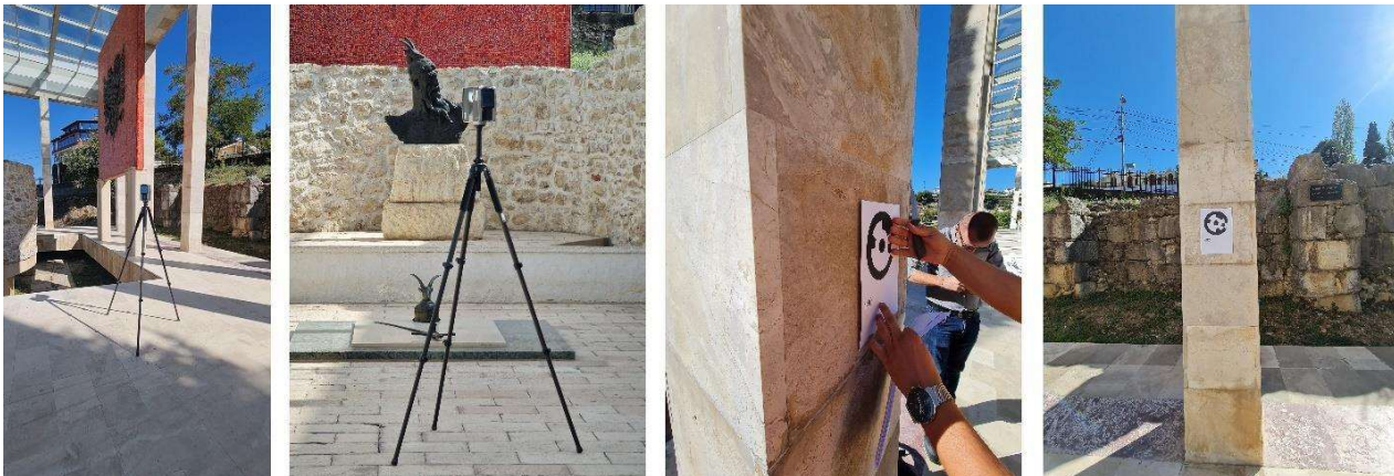
Figure 6 Phases of data acquisition using the laser scanner.
