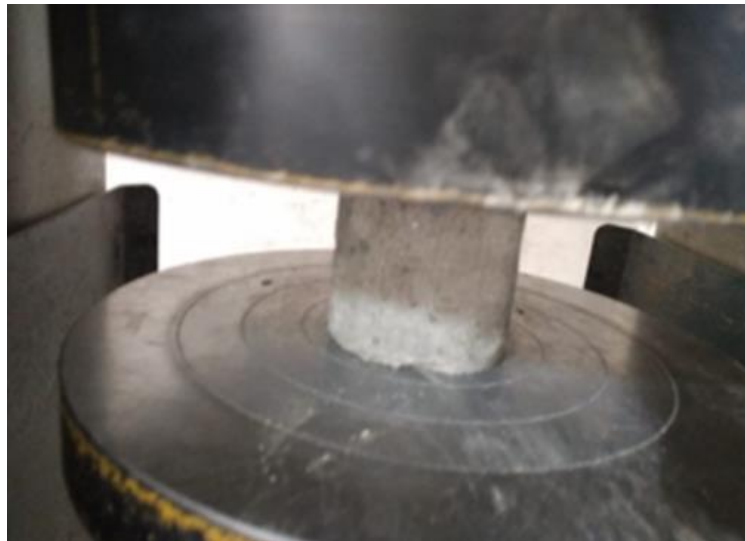
Figure 101: Laboratory test for the concrete sample of 1982 template building
