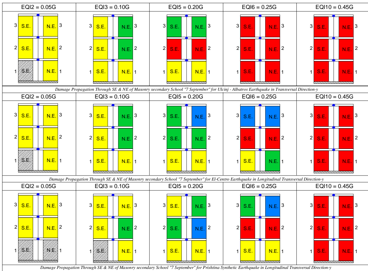
Figure 7. Damage propagation through SE and NE for Building, secondary School, under three earthquake in y-direction
