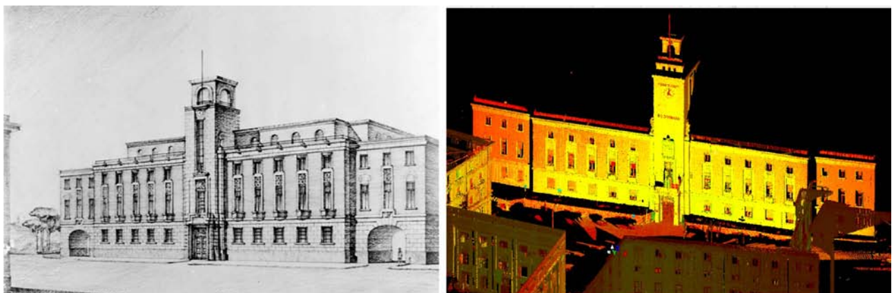
Fig. 11 – 12: Palazzo del Governo in Enna. On the left, the first solution of the project (1935) with the galleries to access the belvedere at the back; on the right, view of the 3D digital survey of the Palazzo del Governo .
