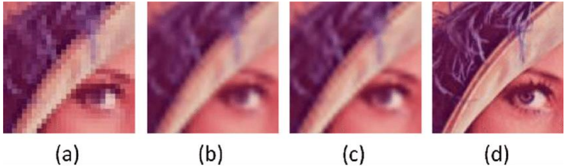
Figure 1. Visual comparison of different interpolation methods. (a) Nearest neighbor. (b) Bilinear. (c) Bicubic. (d) Original HR image (4x) Picture is found at ‘Super-resolution via adaptive combination of color channels’ [5]
