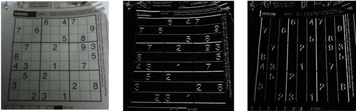
Figure 16. The illustration of both sobel operators Gy and Gx for the detction of edges in the horizontal and vertical direction respectively
