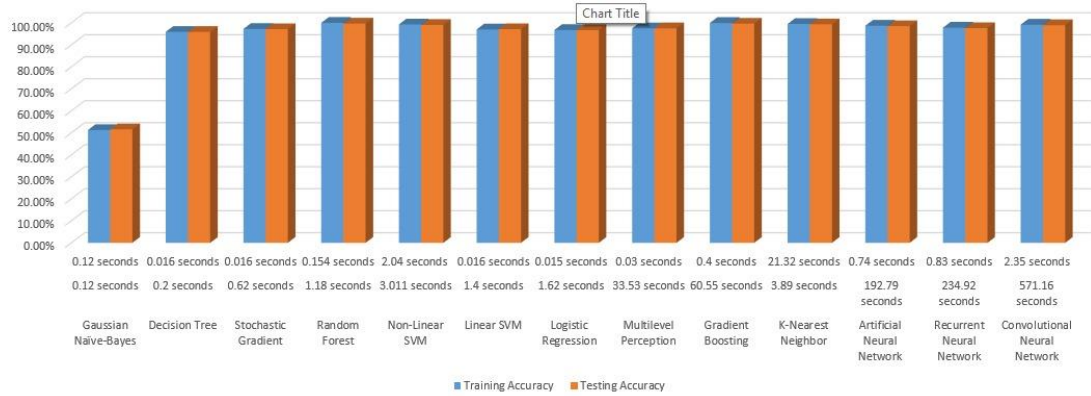
Fig 25: The outcomes of the training and testing methods for the nsl-kdd dataset
