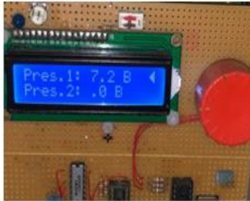
Figure 22. PLC mounted on the system. As you can see in 7.6 Bar with the SET POINT 7.5 only one motor is working with 90% of the power when the pressure drops to 5.0 the motor one reaches the maximum and the second motor starts working.
