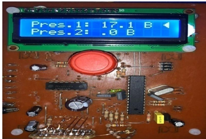
Figure 18. HOME is the section which shows the pressure at the working state. It can easily be mount 2 or more sensors. In this case only one sensor is mounted
