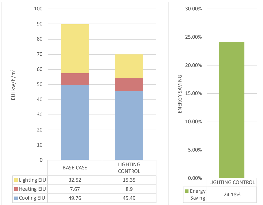
Figure 34. The comparison of Cooling, Heating, and Lighting Energy Use Intensity (EUI) between the Lighting Control Case and the Base Case demonstrates a savings of 24.18%.
