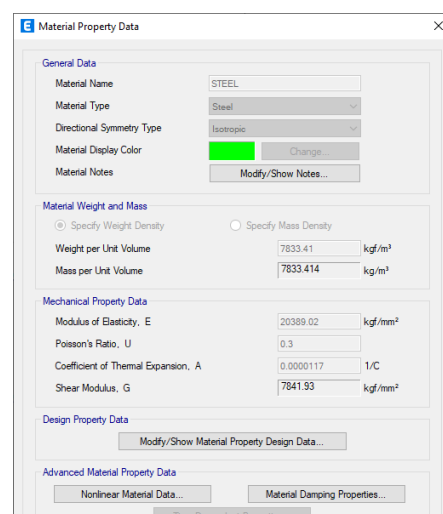
Figure 36. ETABS Material Property Data form -Rebar
