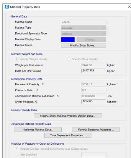
Figure 35. ETABS Material Property Data form -Concrete
