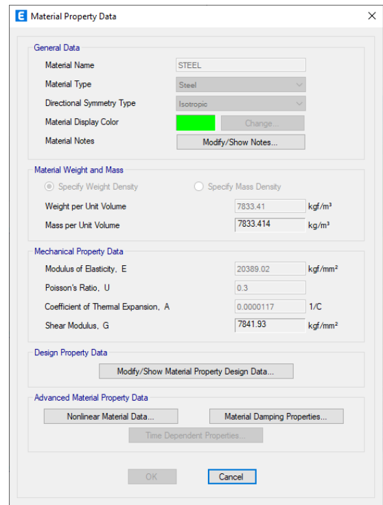
Figure 24. ETABS Material Property Data form -Rebar
