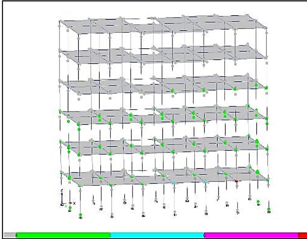
Figure 54. Development of plastic hinges with reference to Figure 53 (the distribution of plastic hinges), for the six-story building
