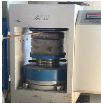
Fig 20 Testing of the solid bricks procedure according to EN 772
