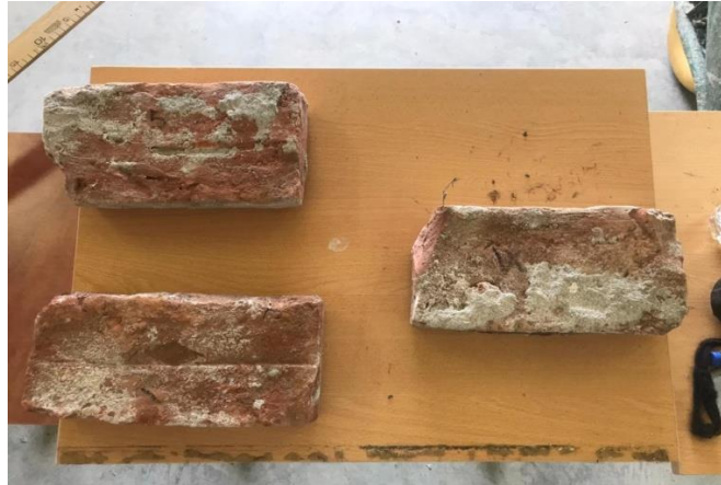
Fig 19 Samples for laboratory tests of bricks from the studied object (Solid bricks 25x12.5x6 mm)
