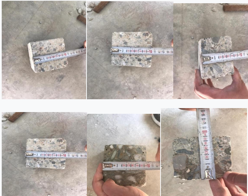
Fig 13. Preparing the concrete samples (Creating concrete cubics )
