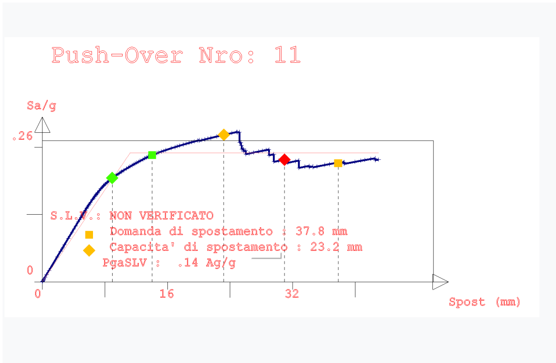
Fig.65 the capacity curves for the limited state of the not collapse SLV (Node 11)
