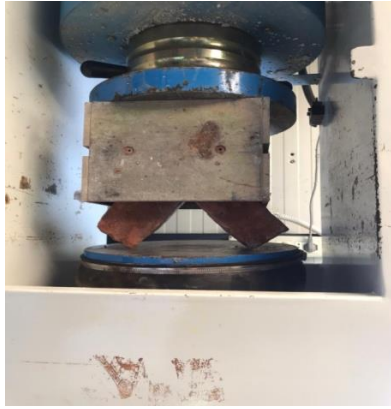
Fig 21 Loading the solid bricks until their failure according to EN 772
