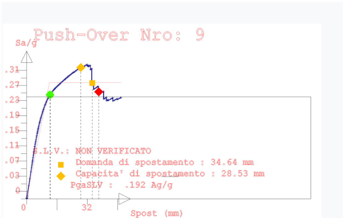
Fig.64 the capacity curves for the limited state of the not collapse SLV (Node 9)
