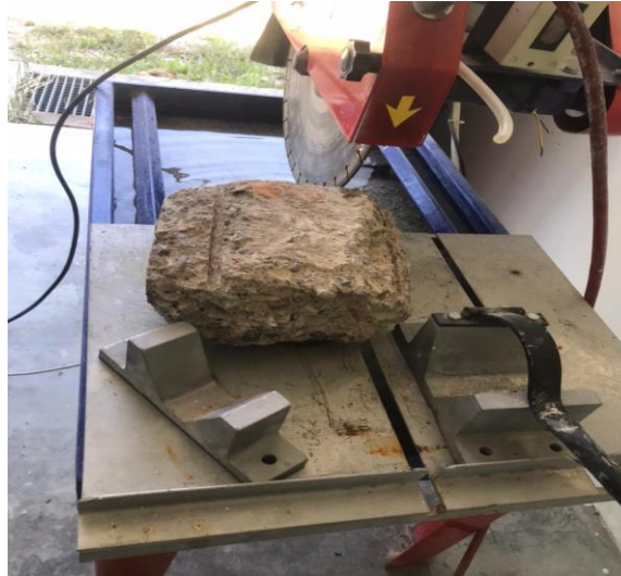
Fig 13. Preparing the concrete samples (Creating concrete cubics )
