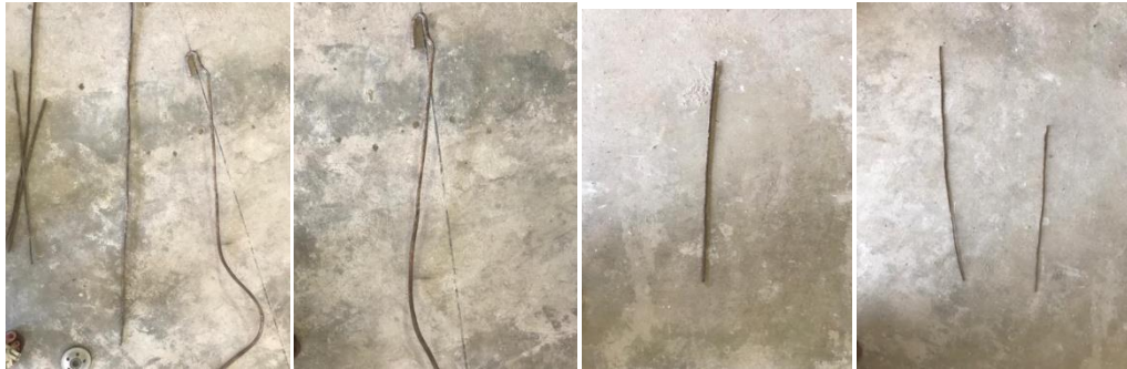
Figure 16 The prepared steel testing element taken from the damaged object
