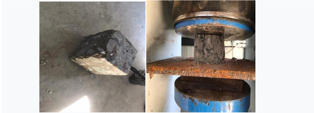
Fig 15. Testing the prepared concrete cubics into the apparatus and measuring the compressive strength
