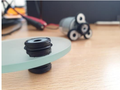
Figure 33 The motor and the diffuser used to realize the rotating diffuser
