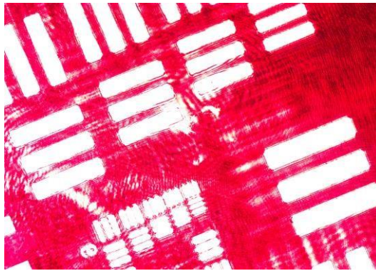
Figure 35 Image with red laser illumination without a diffuser
