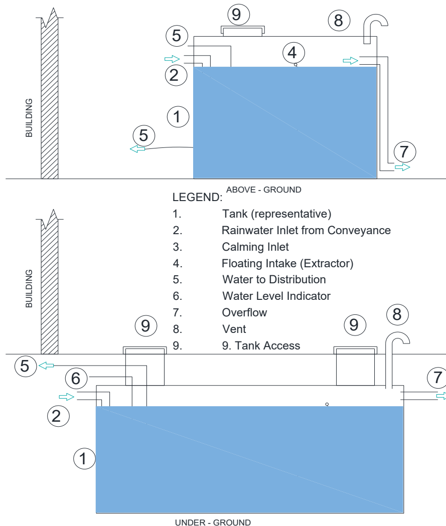
Figure 7. Components of a storage system
