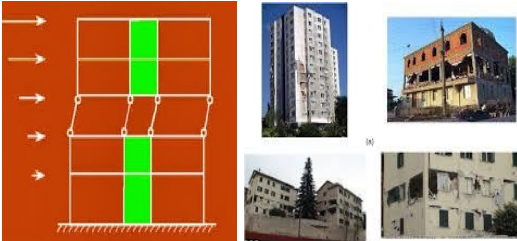
Figure 10. Intermediate soft story scheme. Figure 8. Progressive Collapse of Concrete Frames with Unreinforced Masonry Infill Walls Considering In-Plane/Out-of-Plane. [Khalid M. Mosalam and Selim Günay, 2015]
