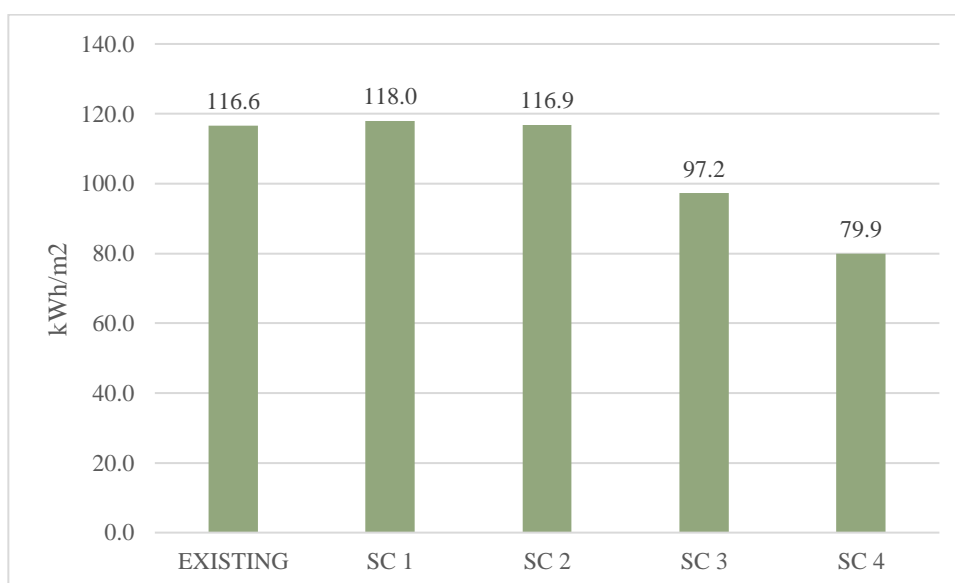
Figure 78 Comparison of total yearly energy demand of the Existing state and SC1 - SC4 for B2.
