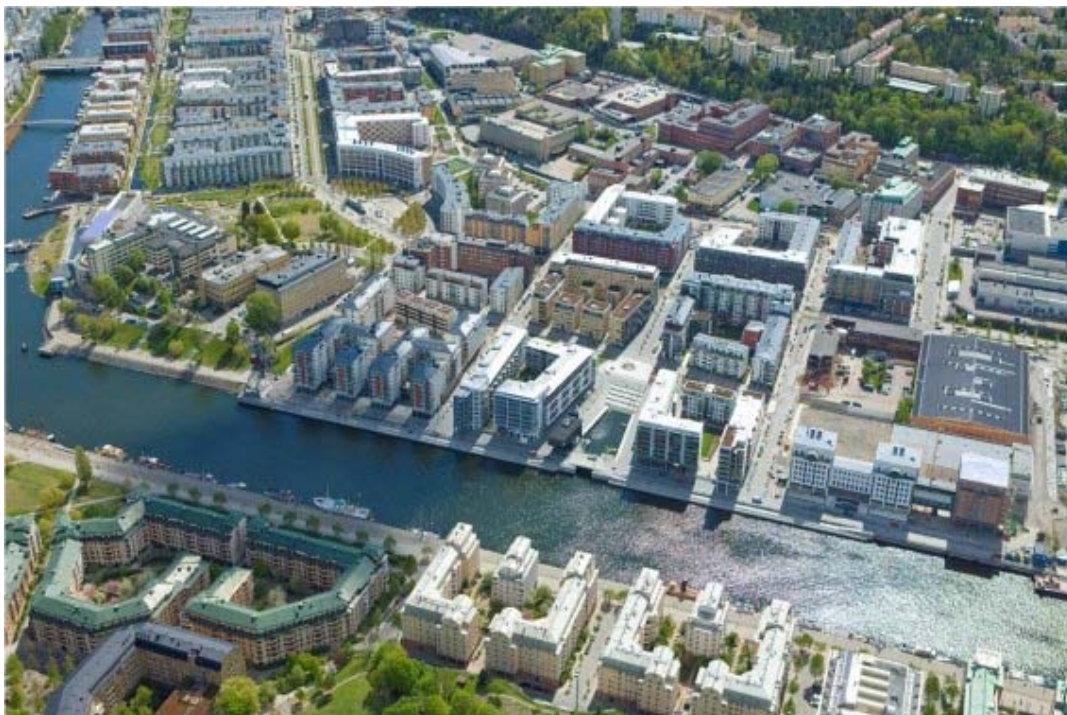
Fig. 2: Hammarby Sjöstad, Stockholm. The residential districts adjacent to the main spine follow a grid structure with a semi-open block form, which allows for maximum light and views as well as providing open access to the courtyards of residential blocks. Most apartments have balconies, terraces and green roofs , which provide overlooking onto the streets, waterfront walkways and open spaces . A network of varied parks, green spaces and walkways runs through the district as well as pedestrian walks, quays and linear parks across the waterfront. The street dimensions, block lengths, building heights, density and usage mix were designed to take advantage of water views, parks and sunlight. Reduce car usage and alternative transportation options at the planning and implementation, the possibilities to sporting and leisure activities, inner courtyard or play area, public spaces, restricted building depths, ecological building materials, solar panels etc. are just a few elements of design code which is preparing in order to support environmentally friendly housing and improving quality of resident lifestyles. Some of the environmental goals for land usage are: 1) open space standard: there shall be at least 15m 2 of courtyard space and a total of 25–30m 2 of courtyard space and park area within 300m of every apartment (equiv. 100m 2 BTA), 2) at least 15 % of the courtyard space shall be sunlit for at least 4–5 hours at the spring and autumn equinoxes, 3) development of undeveloped green public spaces shall be compensated for in the form of biotopes that benefit the biological diversity in the immediate area, 4) natural areas of particular value shall be protected from development.
