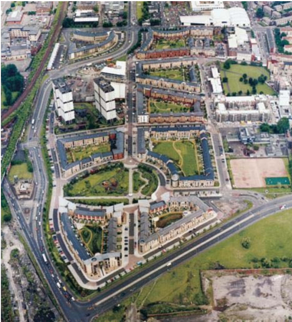
Fig. 3: Crown Street – Glasgow. Each of the residential developments is designed as a perimeter block and set around a communal garden that can be used by the residents. Each home on the ground floor of the blocks also has a small private garden that backs onto the larger communal garden . Each block has been designed by a different architect and features a theme of decoration and street art, either through murals or sculpture, in order to create distinctiveness and a sense of place.
