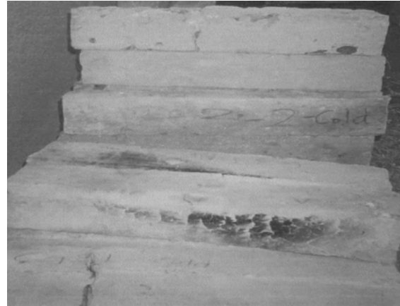
Fig 2 Concrete Beams after firing
