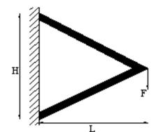
Figure 1 – Two member structural frame
