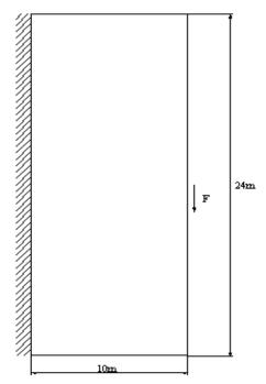
Figure 2 – Design area for two member structural frame
