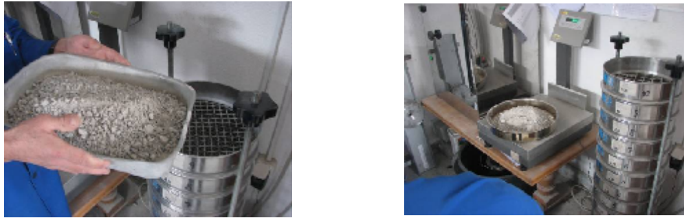
Fig. 11 Process of sieving the recycling aggregate
