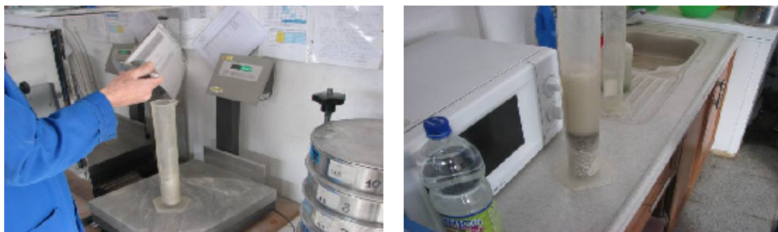
Fig. 7 The process of determination of specific density
