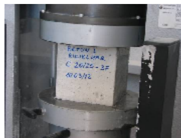
Fig. 20 Examination of recycled concrete
