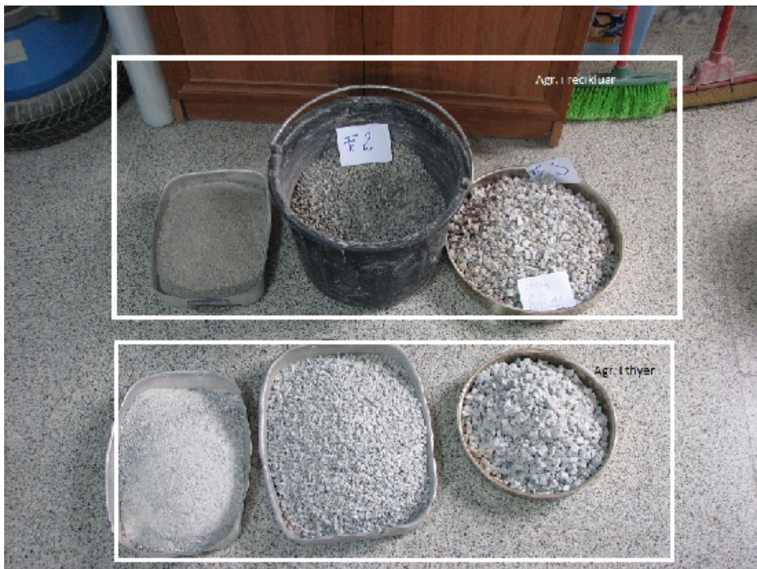
Fig. 9 Visual differences between ordinary and recycled aggregate
