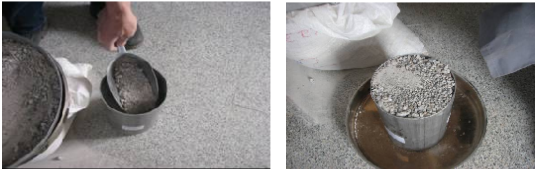
Fig. 6 Determination of bulk density of Recycled aggregate
