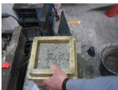
Fig. 17 preparing the concrete samples
