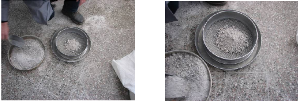
Fig.8 . Manually stifting of recycled aggregate
