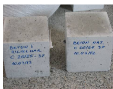
Fig. 18 Ready concrete samples
