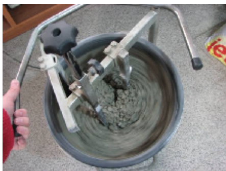
Fig. 15 Mixing of concrete
