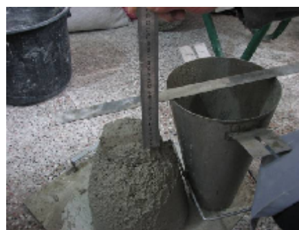
Fig. 16 Slump test ( S-3 plastic concrete)
