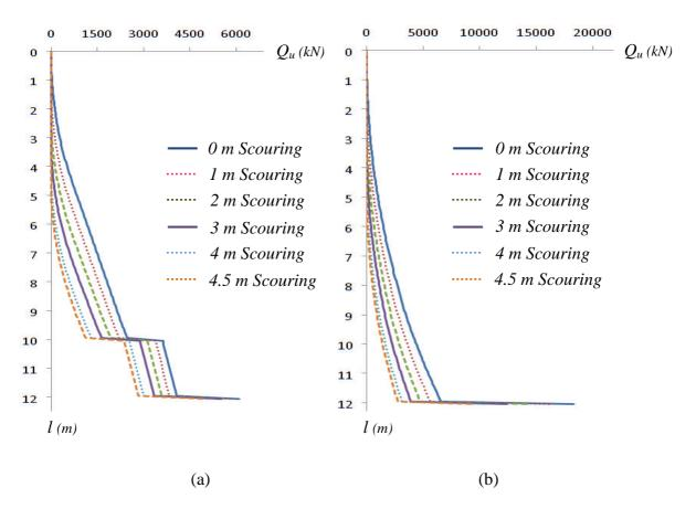
Figure 5. Bearing capacity of piles groups (a) 30cm diameter piles, (b) 100 cm diameter piles.
