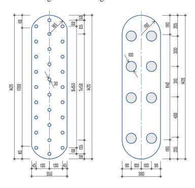
Figure 2. Pile cap view
