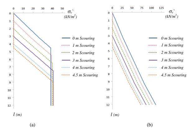
Figure 4. Effective soil pressure distribution, (a) 30cm diameter piles, (b) 100 cm diameter piles.
