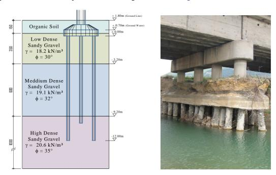
Figure 3. Soil profile and scoring view of pile group
