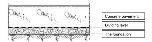
o Pavement based on the slab
