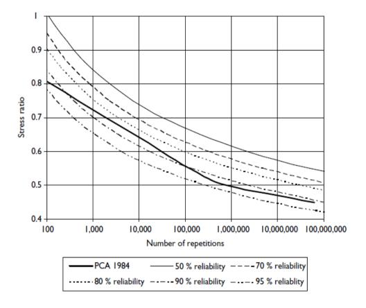
On this graphic, for SR=0.80202, we obtain the number of repetitions. In this case, this number is 100 repetitions. The result is not profitable, so we will increase the thickness, h=30cm. Following the same steps, for h=30cm, we calculate SR=0.612 and determine the number of repetitions (from the graphic) 77500.
