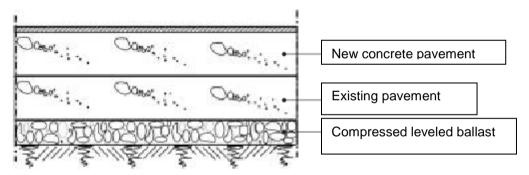
o Pavement based on an isolation layer
