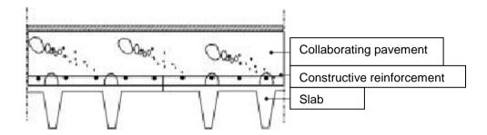
o Pavement based on an existing pavement
