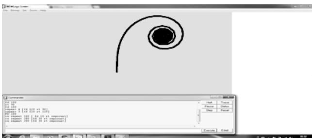
Fig. 5. Logo interface. The shape code in logo is Forward 10, Return right 30, C's Repeat 120 [fd 10 rt repcount]
