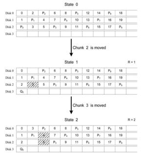
Figure 3. A series of states in data redistribution for RAID-5 scaling from 3 disks to 4. The reordering window is represented by "R".
